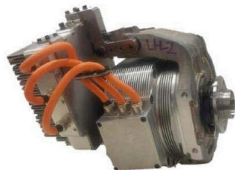
Fig. 13. Air cooled in-wheel drive system developed within the FP7 programme EUNICE project (from Ref. [240]).
